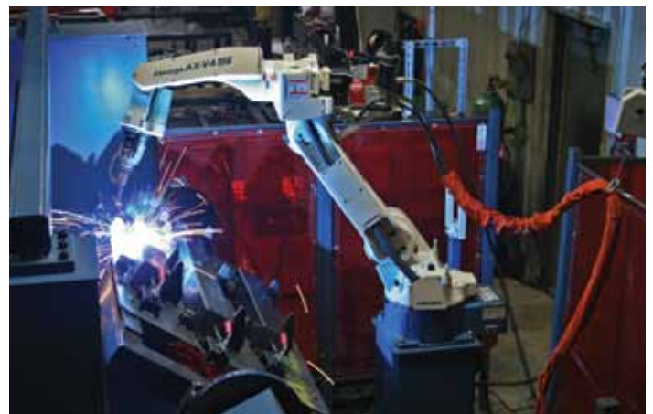
Our Worker Automation welding robots have two rotating positioners and can weld product 40"x84"x550 lbs.
