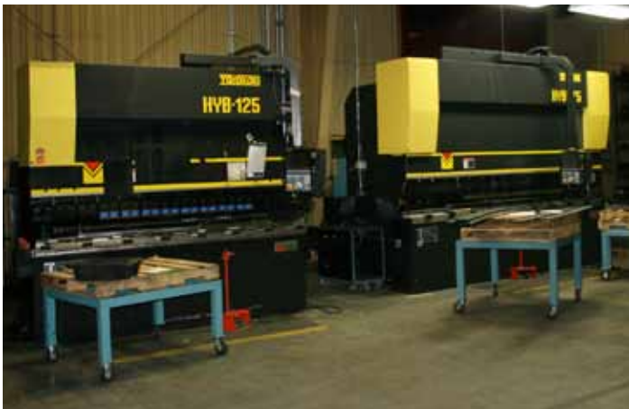
Our 9-axis Toyokoki Brake Presses produce extremely accurate products and utilize Wilson Precision Press Brake Tooling and Express Clamping Systems.
