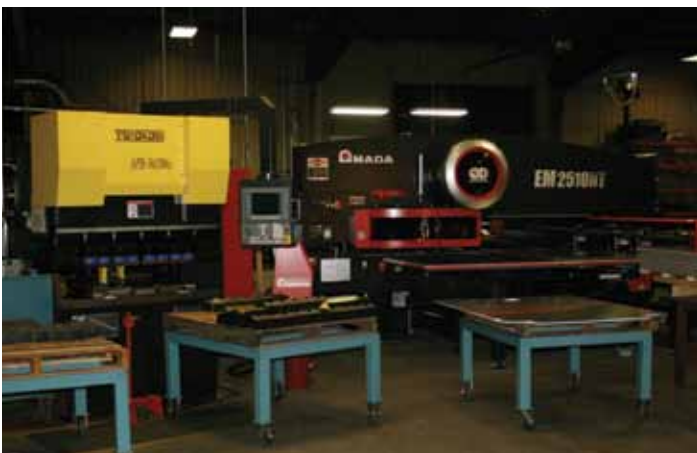
Amada EM2510NT Turret Press and Toyokoki APB Brake cell: In keeping with our 'Lean Manufacturing' philosophy we form parts internal to the turret press machine cycle.
