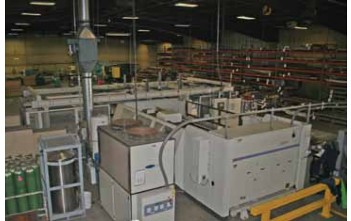
Our 4000 watt Mitsubishi laser can process 1" steel plate, 3/4" stainless steel and 1/2" aluminum up to 60" wide and 120" long.
